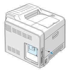
7 Replace the metal cover, as shown below, and tighten the two screws you removed in step 3.
